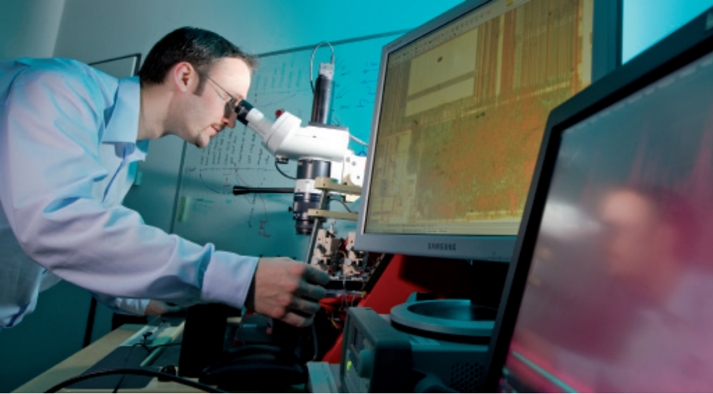
Electro-magnetic emission analysis setup
