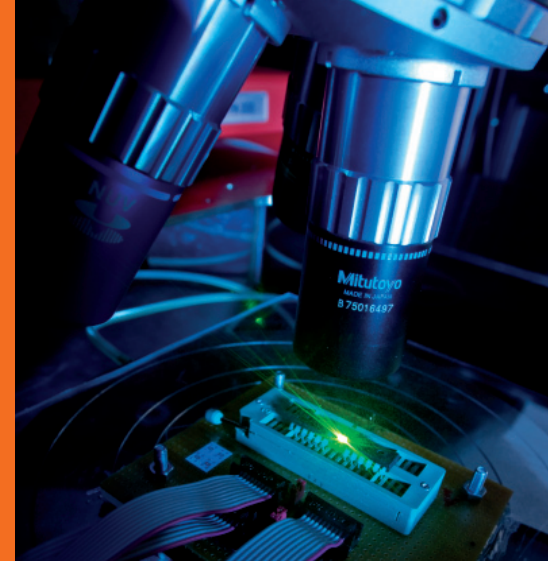
Microcontroller under test in laser station
