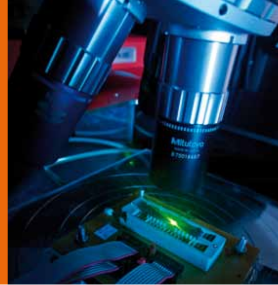
Microcontroller under test in laser station
