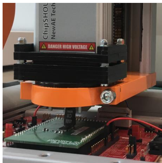
Figure 4.2: Picture of the laboratory setup to reproduce the flash erase suppression attack.
